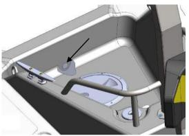
Fig. 7. Recess drainage.
