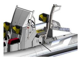
Fig. 12. Ventilation opening of battery.
