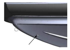
Fig. 6. Bow anchor drainage.
