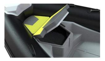
Fig. 34. Bow anchor storage and bow locker.
