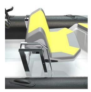
Fig. 41. Helm and passenger SD-26 with pivot seats.
