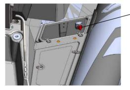
Fig. 27. Battery isolator switch.
