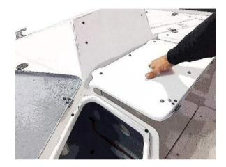
Fig. 45. How the rear sundeck should be installed.
