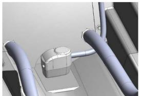
Fig. 5. Bilge pump and its location.
