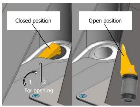
Fig. 3. Cockpit drainage.
