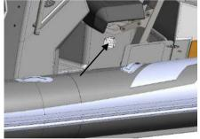
Fig. 10. Ventilation opening on the rear side compartment.
