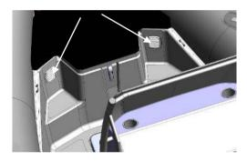
Fig. 9. Ventilation openings on the bow compartment.
