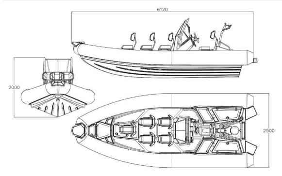
Fig. 70. General view of a boat D600 DRIVE.
