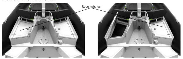
Fig. 53. Rear side rope hatches.
