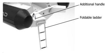
Fig. 13. Foldable ladder and handle for assistance with re-boarding.
