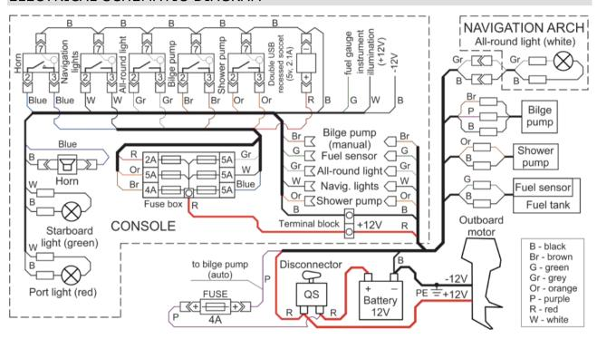
Fig. 73. Electrical schematic diagram.
