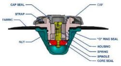
"O" ring and cap seals of the valve can wear out overtime and can be subject to change.
