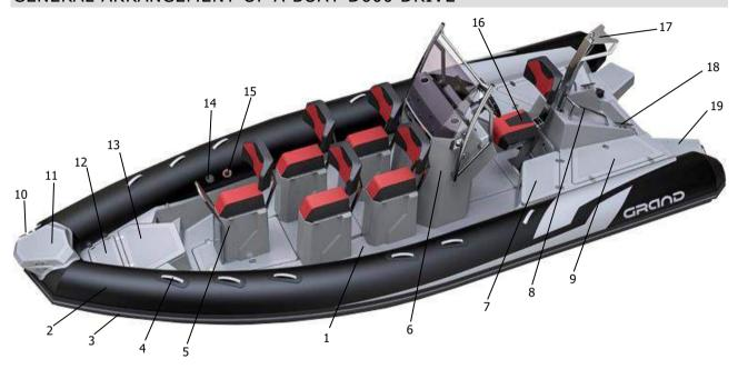
Fig. 66. General arrangement of a boat D600 DRIVE.
