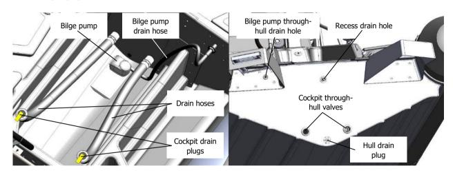
Fig. 2. The drainage system.
