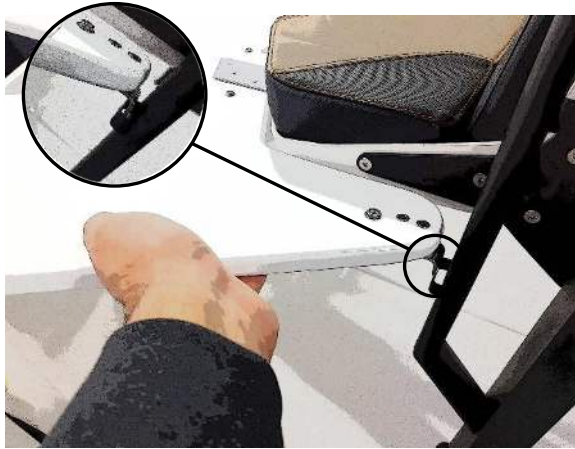
Fig. 49. How the rear sundeck should be installed.
