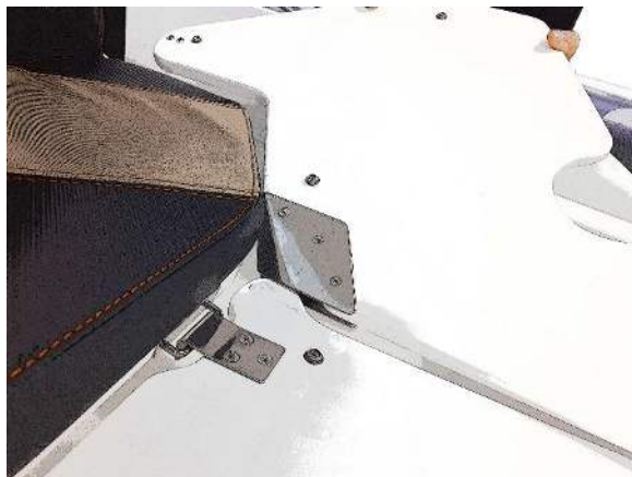
Fig. 48. How the rear sundeck should be installed.
