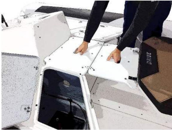
Fig. 47. How the rear sundeck should be installed.
