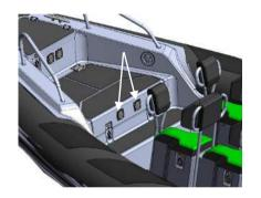
Fig. 11. Ventilation openings on the bow compartment.
