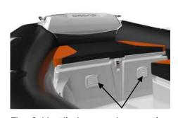
Fig. 6. Ventilation openings on the bow locker.
