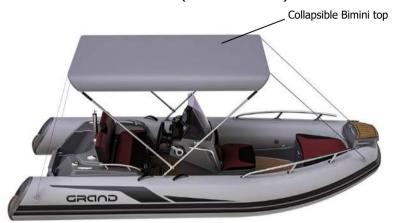
Fig. 34. Collapsible Bimini top.
