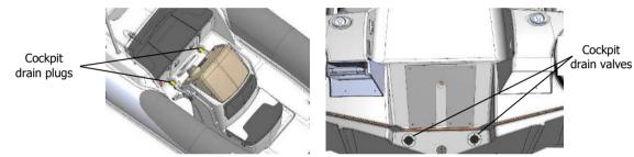
Fig. 2. Cockpit drainage.
