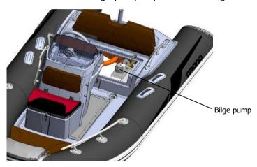
Fig. 4. Bilge pump and its location.
