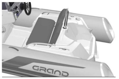
Fig. 32. Rear lockable seat with cushion and seat back.
