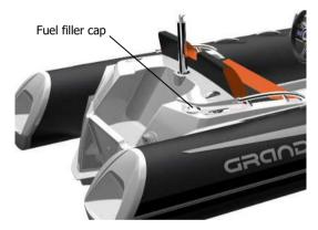
Access to the top part of the fuel tanks, as well to the connections and fuel sensor is provided through the hatch located on the deck and fixed by the screws. To get the possibility to unscrew and then open the hatch, the steering console should be removed.
