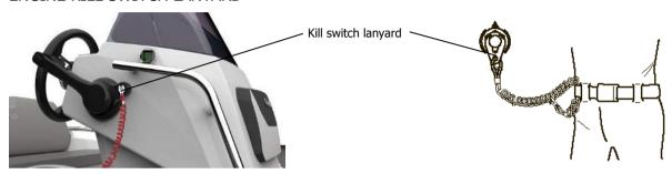
Fig. 22. Engine kill switch lanyard.
