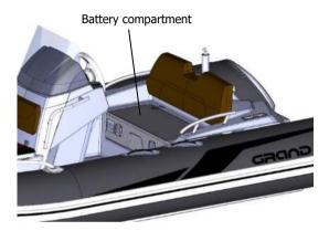
If you don't use the boat/battery for long time or during winter period, recharge the battery at least one a month to extend the battery life.
