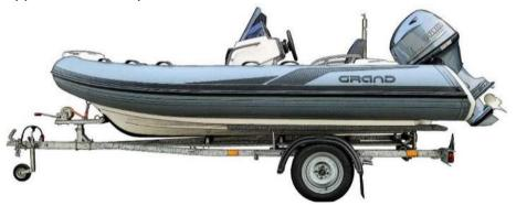
The boat is designed to be transported with an inflated tube.
