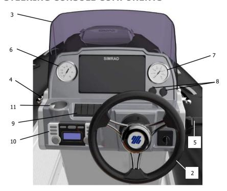
Fig. 44. Steering console components (see the list on the next page).
