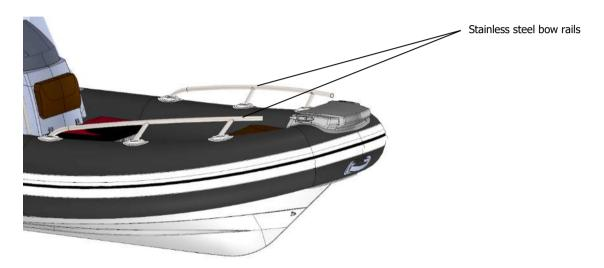
Fig. 33. Stainless steel bow rails.
