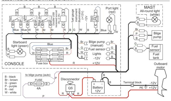
Fig. 46. Electrical schematic diagram.
