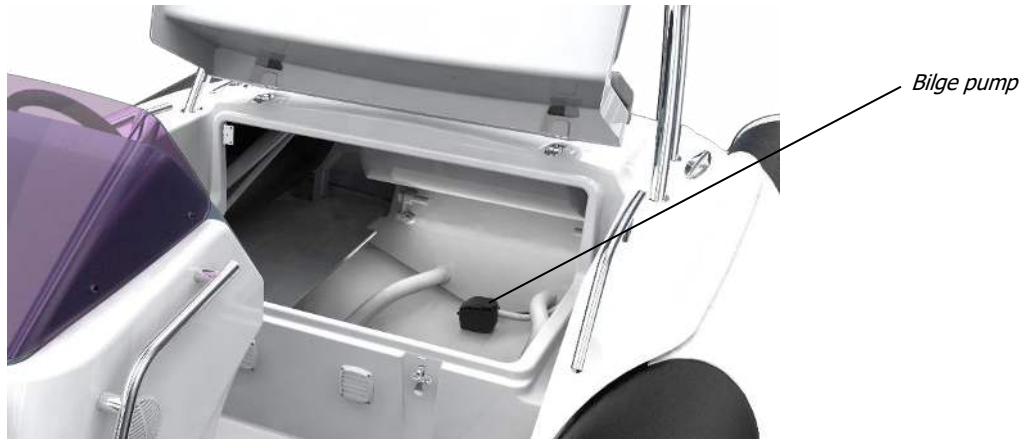
Fig. 4. Bilge pump and its location.
