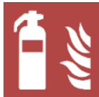
Fig. 9. Symbol of designated place of portable fire extinguisher.
