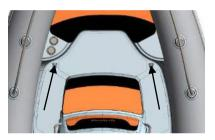
Fig. 28. Bow lifting eyes, 2 positions.
