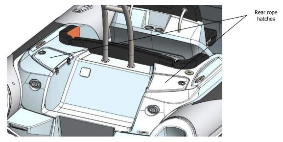
Fig. 32. Two rear rope hatches.
