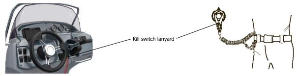
Fig. 23. Engine kill switch lanyard.
