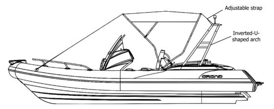
Fig. 39. Installation of Bimini Top on a boat with inverted U-shaped arch.
