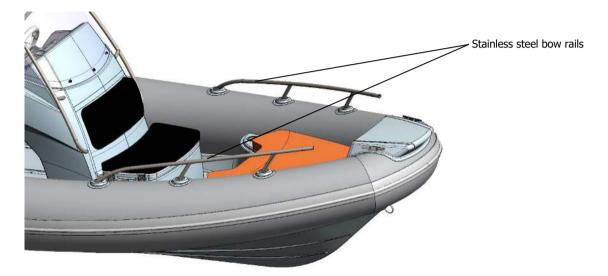
Fig. 36. Stainless steel bow rails.
