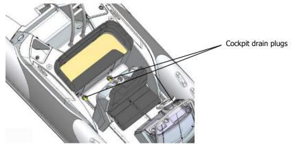
Fig. 3. Cockpit drain plugs.
