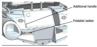
Fig. 10. Foldable ladder and handle for assistance with re-boarding.
