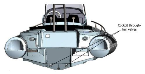
Fig. 2. The cockpit drain valves.
