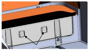
Fig. 7. Ventilation openings on the rear storage.
