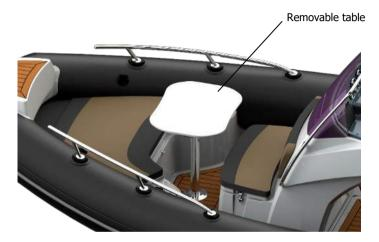
ASSEMBLE A TUBULAR PYLON AND A TABLETOP, AND THEN INSERT IT INTO THE TABLE HOLDER.
