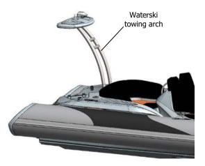
Fig. 43. Waterski towing arch with GRP top.
