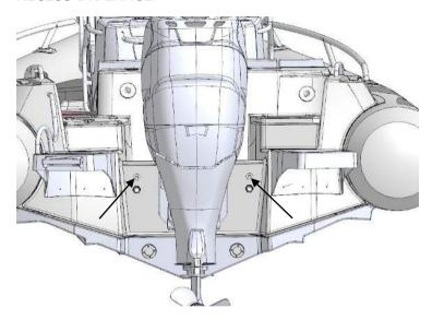
Fig. 6. Recess drainage.
