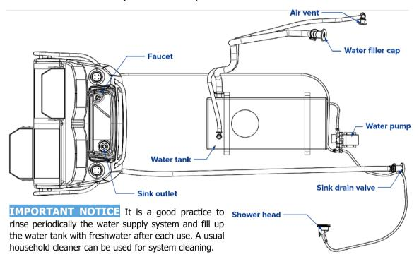
Fig. 45. The water supply system.
