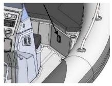
Fig. 9. Ventilation opening on the bow compartment (starboard).
