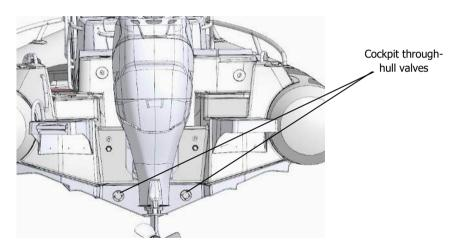
Fig. 2. The cockpit drain valves.
