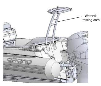
Fig. 42. Waterski towing arch.
