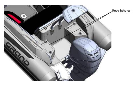
Fig. 37. Rear side rope hatches.
