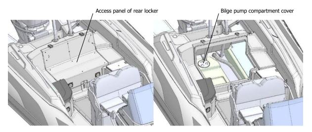
Fig. 5. Location of a bilge pump in rear locker.
