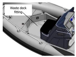
Fig. 51. Location of the waste deck fitting.
