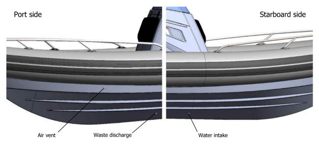
Fig. 49. Wastewater system. Location of air vent, water intake and waste discharge fittings.
