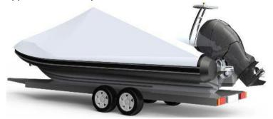
The boat is designed to be transported with an inflated tube.
