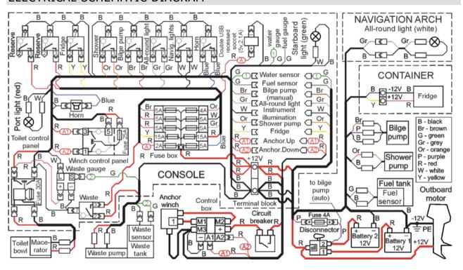
Fig. 65. Electrical schematic diagram.
