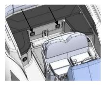
Fig. 10. Ventilation openings on the rear side compartment.
