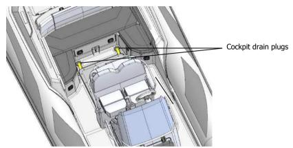
Fig. 3. Cockpit drain plugs.
