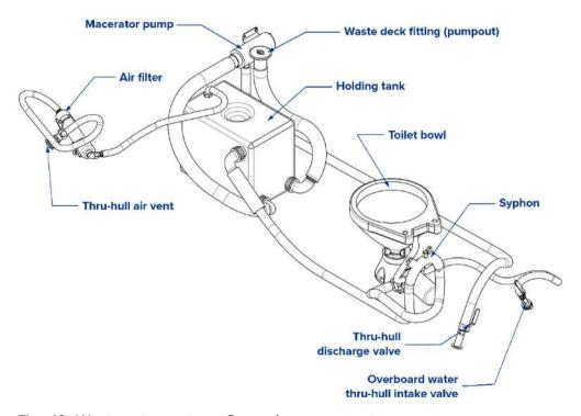
Fig. 48. Wastewater system. General arrangement.
