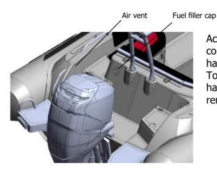
Access to the top part of the fuel tanks, as well to the connections and fuel sensor is provided through the hatch located on the deck and fixed by the screws. To get the possibility to unscrew and then open the hatch, helm and passenger double seat should be removed.
