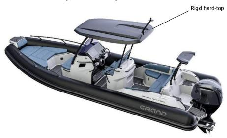
Fig. 53. Rigid hard-top (view A).
