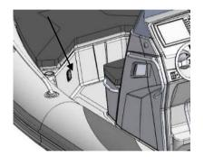
Fig. 8. Ventilation opening on the bow compartment (port side).
