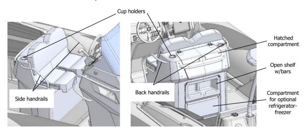
Fig. 34. Helm & passenger seat / bolster with functional wet bar.
