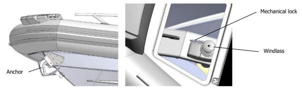
Fig. 56. Windlass and anchor.
