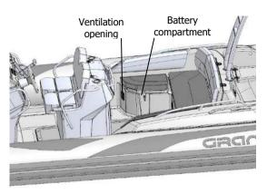
If you don't use the boat/battery for long time or during winter period, recharge the battery at least one a month to extend the battery life.
