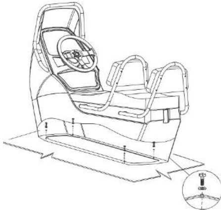
Fig. 7. Installation of steering console CS-03.
