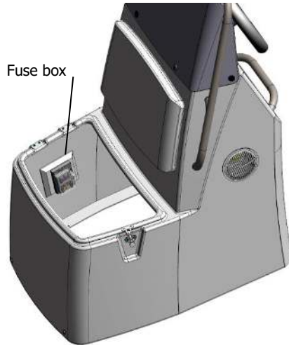
Fig. 21. CL-14. Fuse box location.
